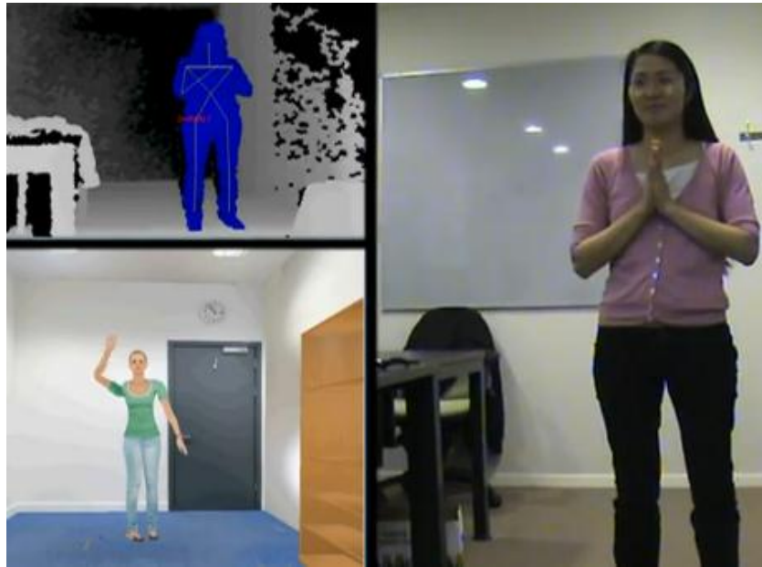
Figure 2. Prototype of the gesture translator for Western and Asian greeting gestures. On the right a participant's bow gesture, on the upper left the recognized participant and its joints in a typical frame and on the bottom left the translated gesture onto an avatar.
