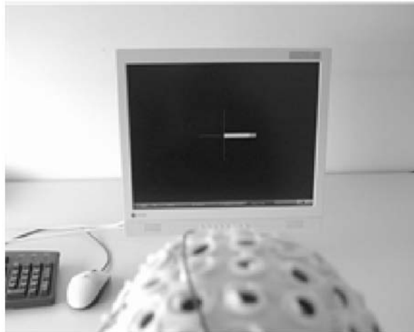
FIGURE 3. “Traditional” BCI in front of a monitor: the arrow on the red cross indicates to the participants whether they should imagine moving their hand or their feet. Participants need to keep concentrating on this thought as long as the arrow is displayed, for 4.25 sec. If a classifier is already available, the white bar provides immediate and continuous feedback for 4.25 sec.
