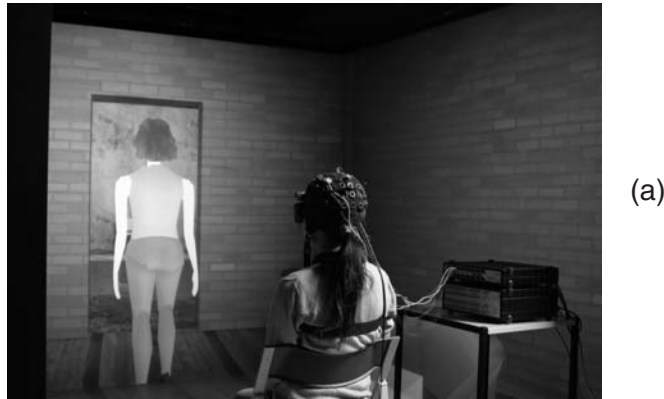
FIGURE 5. (a) A female participant and her avatar in the virtual room. The participant is connected to the BCI equipment, inside the Cave-like system. (b) A male participant with the male avatar, in the same setting.
