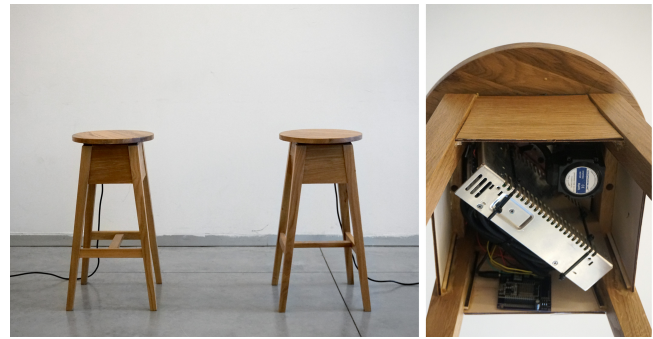
Figure 2: Left: A pair of robotic bar-stools. Right: The motors, gear, and microcontroller hidden within the inner side of the bar-stools
