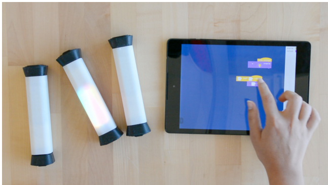
Figure 7. The Scratch-based research platform used to select an animation feedback in one of the Nodes devices.
