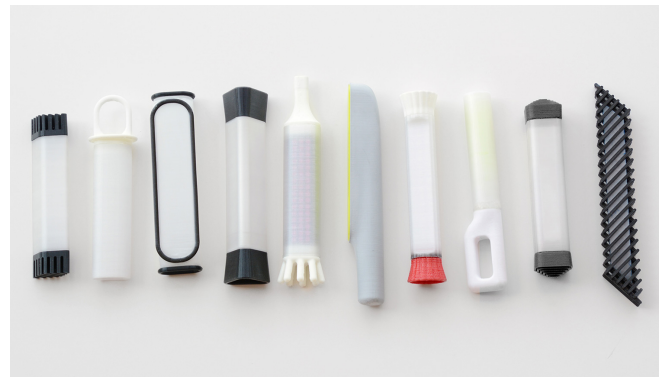
Figure 2. Selection of 3D printed prototypes inspired by the shape of a "stick" and tested for robustness.
