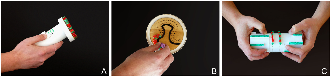
Figure 1: The TUI low fidelity prototypes (A-flashlight form; B-coin form; C-rotation object), each embodies the COS psychological concepts in a different way. The adult holding hand is added for scale and interaction context.
