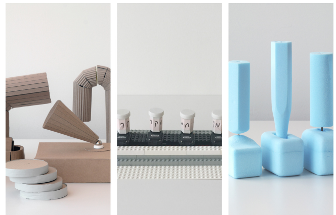
Figure 2. Low-fidelity prototypes made of cardboard, Lego and blue foam used during the design process to validate the form factor with our target users.
