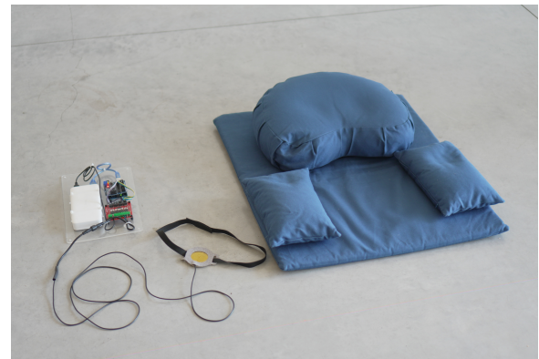
Figure 6: The experimental setting was a quiet room with a meditation rug, meditation sitting pillow, two optional supporting pillows for the legs, and the targeted warmth wearable.
