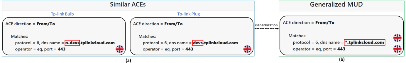
Figure 5: MUDs Comparison (a) and generalization (b) of two different devices of the same manufacturer
