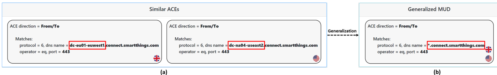
Figure 9: Two similar ACEs from the MUDs of SmartThings hub in two different locations: US and UK. MUDIS created a generalized ACE in which the endpoint is *.connect.smarththings.com , all other parameters remain the same.
