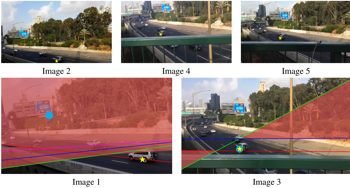
Figure 5.5: Example results of finding correspondence in dataset a2. The top row of images are the given correspondences, the remainder of the images show the chosen correspondences. Correspondences selected using TERs are shown as yellow stars while those selected without are cyan circles. Note: images are labeled based on their order in time but presented in order, of best nearest neighboring matches as selected by the TER algorithm.
