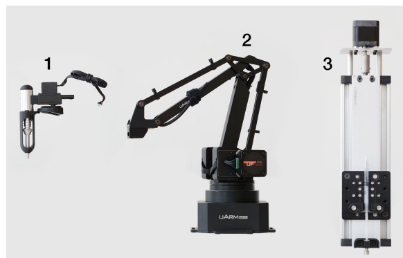
Figure 2. 1. The custom-made liquid handling attachment. 2. the uArm Swift Pro robotic arm. 3. The linear actuator-syringe pump.
