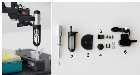
Figure 3. Closeup of the custom-made liquid handling attachment extracting bacterial culture from a tube (left) and disassembled (Right). 1. pipette shaft. 2-3. 3D printed parts for tip displacement. 4-5. 3D printed adapters. 6. uArm end-effector.
