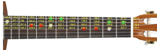
Figure 4.6: The fundamental frequencies of the standard guitars. The pairs of red and green dots mark a pair of indistinguishable notes. Marked with white dots are notes whose fundamental frequency is within the noise range. Frequencies 233.1 and 246.9 are marked as indistinguishable although both their f_0 and h_2 are within the noise range, which practically makes the undetectable.
