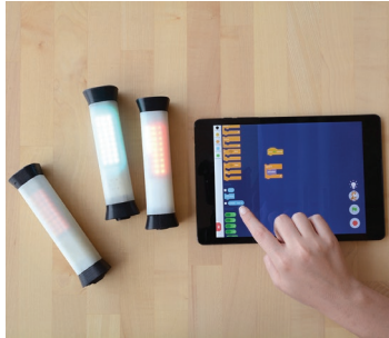
Figure 1: The Tablet runs a Scratch-inspired coding platform, and communicates with the Node devices via Bluetooth Low Energy (BLE). Code is converted into a set of events, and are sent to the Nodes. When an event occurs, the appropriate sensor data is sent back to the tablet, is evaluated, and the appropriate feedback is selected and sent back to the Nodes, generating feedback for the user.
