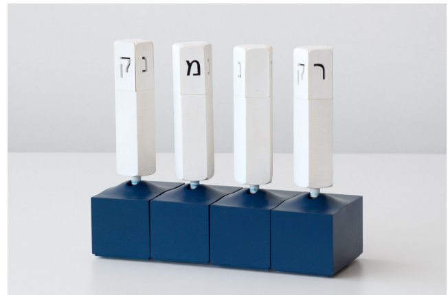
Figure 1: The actuated-interface (extended from [44]), designed as an anagram game with four pillars, each with four Hebrew letters, for both user and system to construct words.
