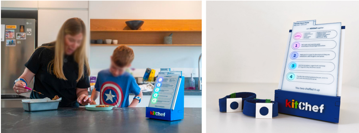
Figure 1: Kitchef: A smart recipe box and a pair of wristbands to motivate parents and children to cook together. Every recipe includes distinct steps, clearly indicated by illuminated hollow circles. These circles light up each time the parent and child attach their wristbands, signifying the completion of a cooking step.
