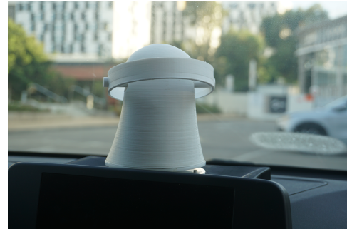
Figure 1: A robotic object for providing social cues and enhancing AV passengers' sense of safety and trust.
