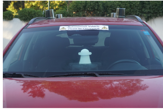
Figure 4: The vehicle modified with objects simulating LIDAR sensors on the roof and large warning stickers
