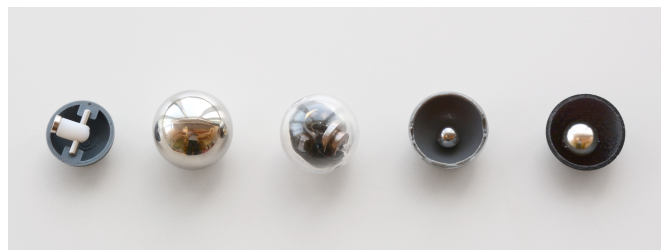
Fig. 4. Various rolling balls designed and tested with the Greeting Machine, spanning a variety of external materials, internal rolling constraints, and ferromagnetic components.
