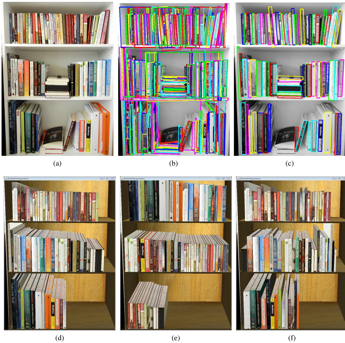
Figure 5.4: Book spine segmentation and reorganization results. a) Original image, b) PR candidates, c) final segmentation results, d) reorganization by height per shelf, e) reorganization by height for all shelves together, f) reorganization by width per shelf.
