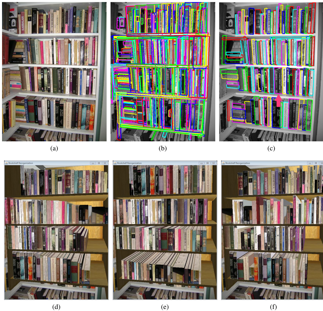
Figure 5.7: Book spine segmentation and reorganization results. a) Original image, b) PR candidates, c) final segmentation results, d) reorganization by height per shelf, e) reorganization by height for all shelves together, f) reorganization by width per shelf.
