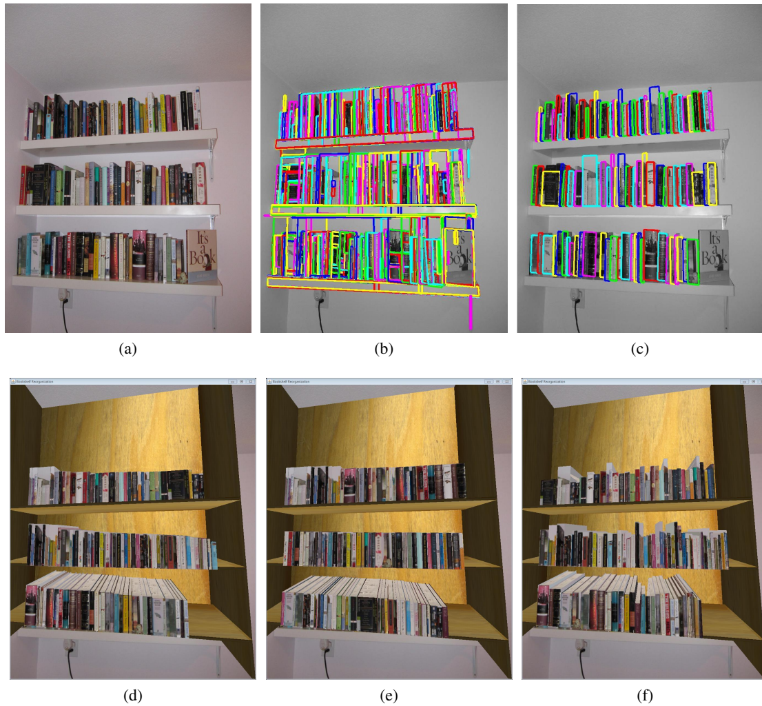
Figure 5.14: Book spine segmentation and reorganization results. a) Original image, b) PR candidates, c) final segmentation results, d) reorganization by height per shelf, e) reorganization by height for all shelves together, f) reorganization by width per shelf.
