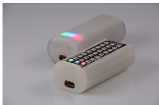
Figure 6: In order to increase the potential for social play among children we designed a robust case that affords holding rather than wearing.
