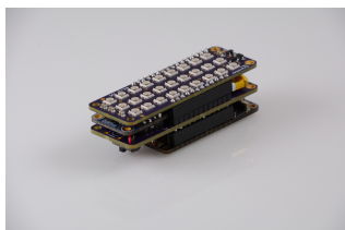
Figure 2: Sensor-based hardware device using the Adafruit Feather (an Arduino clone with built-in Bluetooth support) and an acceleration sensor. We designed a custom display using three columns of 9 LEDs each, based on the metaphor of an abacus: 9 units, 9 tens, and 9 hundreds.
