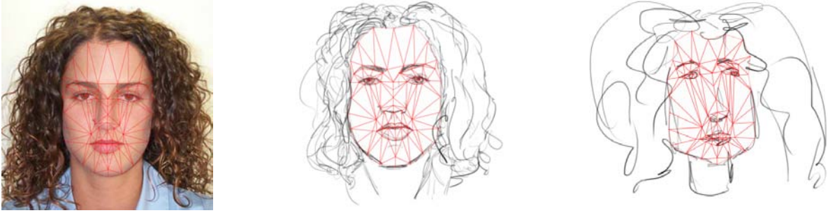
Figure 3.1: Examples of fitting the mesh to the photograph and sketches in various levels of abstraction. The mesh includes eyes, mouth, nose and eyebrows as the important features for face recognition [30].
