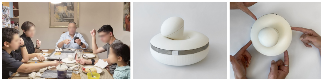
Figure 1: Left: Family at dinner time with the TUI in the middle; Middle: The spinning top TUI showing the base and the rotating top; Right: To stop the rotation, all family members are invited to touch the TUI’s base, reflecting a moment of togetherness (Photos were taken with consent).
