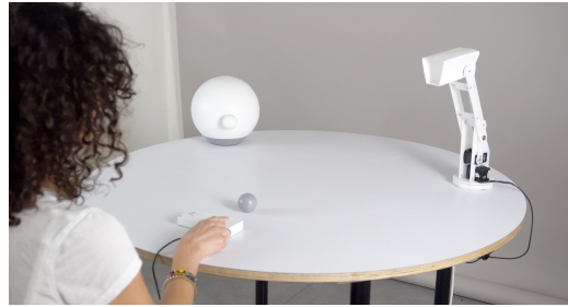
Figure 1: Robot-Robot-Human Interaction. A physical adaptation of the Cyberball paradigm, designed to measure the effect of ostracism by non-humanoid robots.
