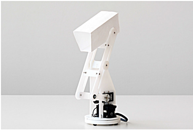
Fig. 1 The robot used in the study (previously published, used with permission; Hoffman et al. [66]) is a simple 2 Degree-of-Freedom non-humanoid robotic object, capable of performing several gestures, including Gaze, Lean, and Nod
