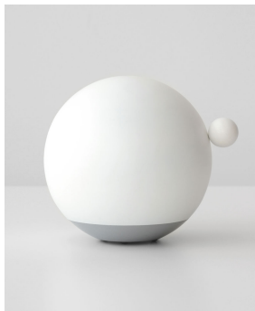
Figure 1: Non-humanoid robot in the form of a small ball rolling on a larger dome. Taken from Anderson-Bashan et al. (2019) [1].
